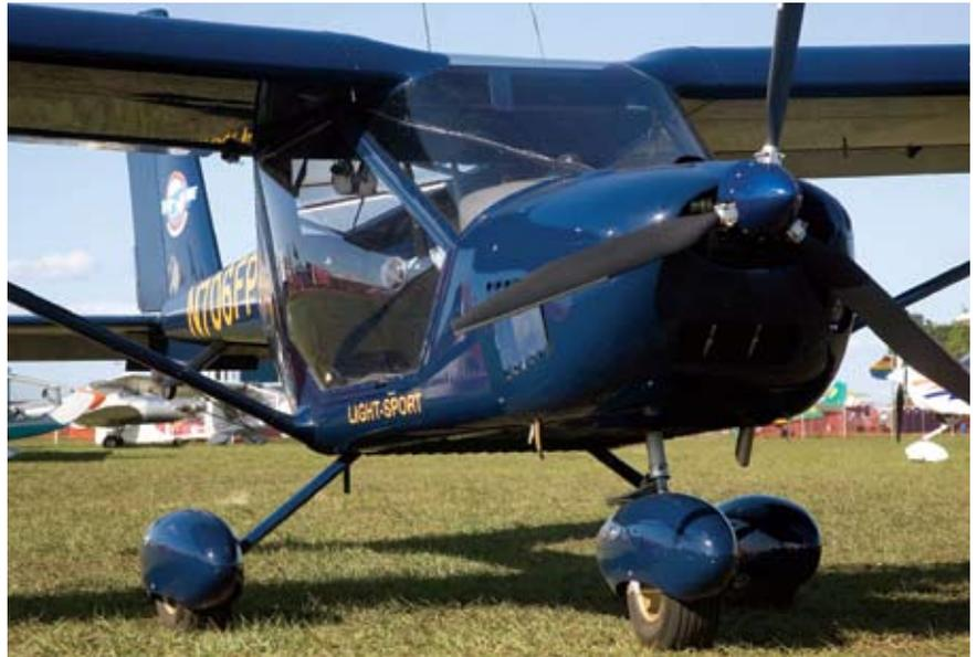
The tri-gear sits low to the ground, making entry and egress easier. Responsive nosewheel steering and differential brakes make the aircraft easy to maneuver on the ground.
